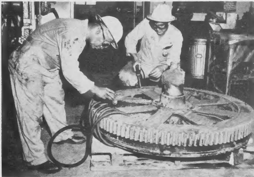
THE MAGNAFLUX operation is carried on in an area outside the EIG lab which is adjacent to the metal trades location. The convenience of the lab's new location presents itself when heavy pieces in the main shops need special EIG attention.
